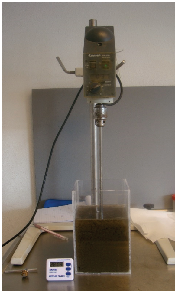
Figure 6.12 Experimental setup for the FSS test. An activated sludge sample is stirred for 30 min in a square flocculation jar (photo: E. Torfs).
