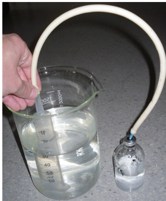
Figure 4.4 Measurement of the volume expansion due to the pressure build-up that is caused by the salting-out of the dissolved gases (photo: van Dongen, 2015).
