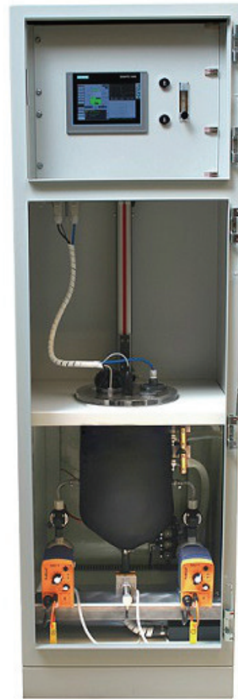
Figure 3.21 Example of a commercial version of a LFS principle-based respirometer using the setup depicted in Figure 3.20. In the middle is the thermostated vessel and at the bottom, left and right, pumps for wastewater and calibration addition (photo: Kelma NV).
